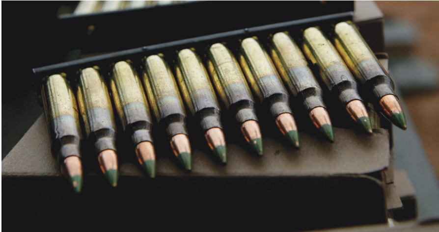
Figure 2.12 Example of 5.56x45mm M855 "Green Tip" cartridges on stripper clips. Note the annealed casing neck. (U.S. Marine Corps image; photographer Cpl. Lydia M. Davey, USMC.)
